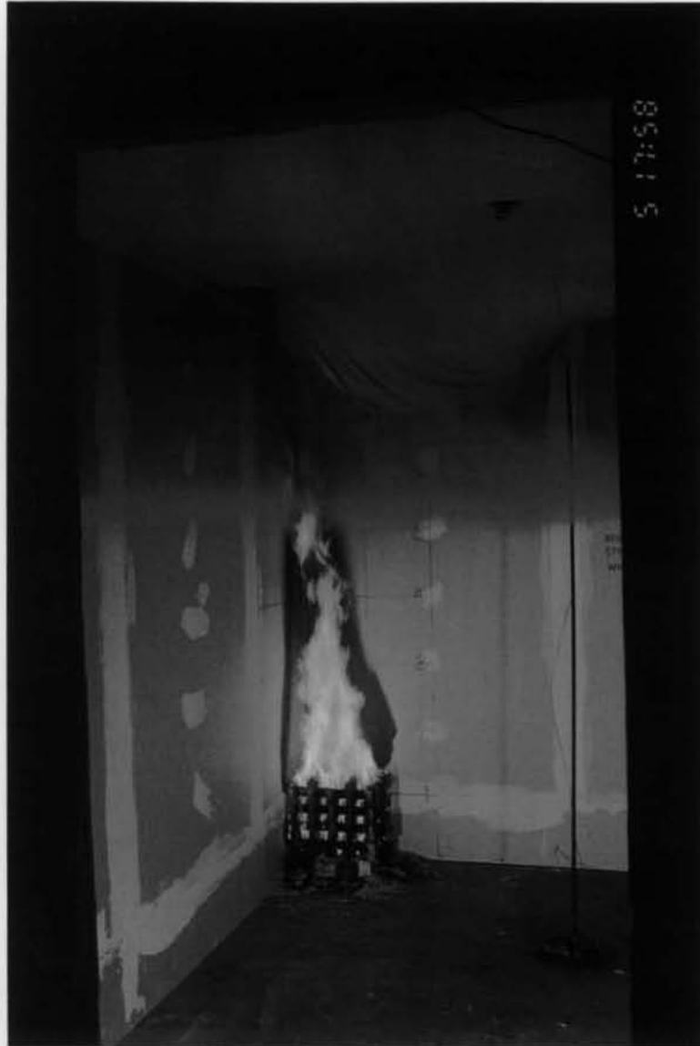
Figure B-7. Room Interior at Approximately 6 Min into Fire Exposure. Reinforced PVC Membrane Is “Hanging Down” Approximately 18 In. (6½ Ft from Floor).
